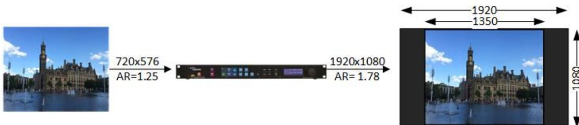
**Full Screen:** The input image is scaled to completely fit the display area without preserving the aspect ratio of the source. This will cause distortion but no black areas will be visible. Example:
