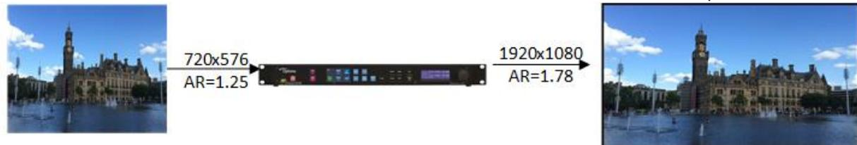
**Crop:** The input image is scaled to completely fit the display area while preserving the aspect ratio of the source. Portions of the input image on the top/bottom or left/right will be cropped out of the output image. Example:
