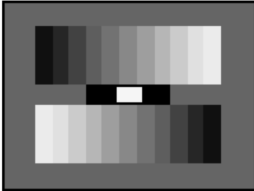
Figure 21 - a Greyscale Test Pattern with correct Gamma. Note all 11 steps of grey can be discerned.
