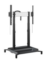
The RISE 5108 motorised display lift floor stand is suitable for displays of up to 86" with a maximum weight of 120kg. The lift raises the display smoothly, quickly, and safely at a speed of 80mm/s with QuickRise™. With a 980mm travel range the lift is suitable for both very low and high positions.
