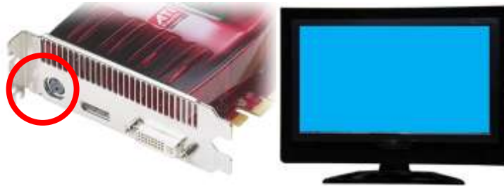
Figure 3: Graphics Card with Stereoscopic connector and 120 Hz monitor with 3 ms delay. In this case the stereoscopic signal may need to be delayed to match the delay of the monitor.
